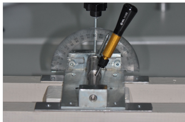
Figure 3. Mini screw application stand and angular apparatus
