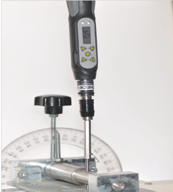
Figure 4. Maximum insertion torque measurement
