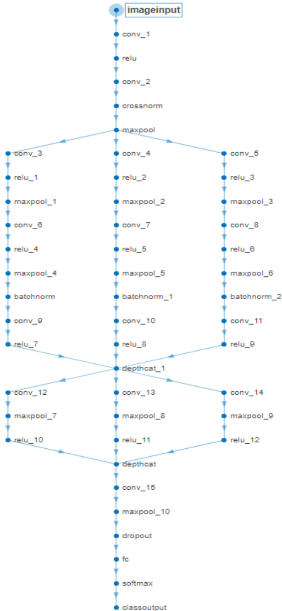
Figure 4. Network design of the proposed model
