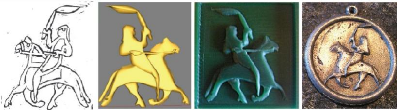
Figure 3: From left to right: An outline of the original wood carving from the Lyngen region of Norway. A 3D model of it. A model made of wax. Final silver jewelry item (Vilbrandt et al., 2011).
