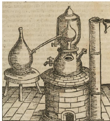
Figure 25. Illustration of distillation apparatus by Vlstadio Patricio (Vlstadio Patricio, 1528, p. xiv).
