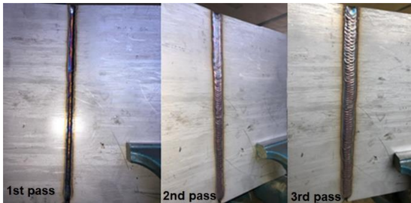
Figure 2. Application of the welding process to plates.
