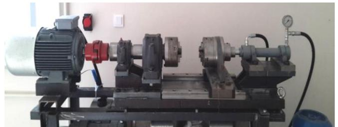
Figure 1. Friction Welding Machine Used in the Experiment
