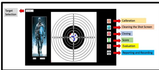
Figure 7. The Capabilities and Interface of the Developed Software
