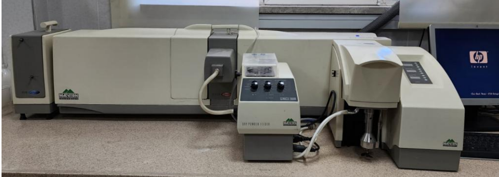
Figure 1. Malvern Mastersizer 2000 particle size analyzer instrument
