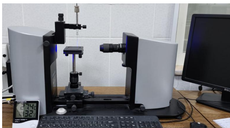
Figure 3. One Attension theta optical goniometer used for water drop contact angle measurement
