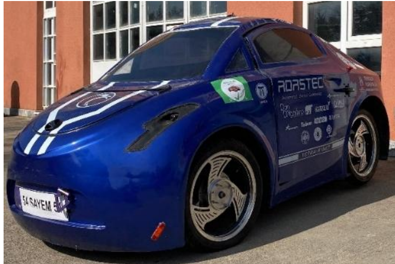
Figure 18. EV with BLDC motor mounted
