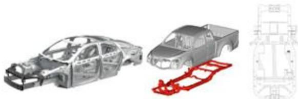
Figure 3.9 Vehicle floor structure design (Left: Monocoque body, Center: Body-on-frame, right: Skateboard architecture) [12,46,47]
