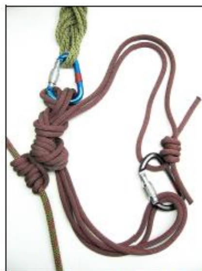
Figure 2. The Munter Mule, consisting of a Prusik Knot on the main line and a Munter Hitch secured with an Overhand Slip Knot and a backup knot. The slack loops are linked for additional security.
