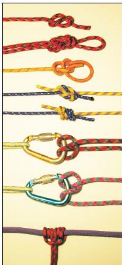
Figure 1. Examples of common climbing knots, from top to bottom: Figure Eight Stopper Knot, Figure Eight Loop, Bowline, Flemish Bend, Double Fisherman's Knot, Clove Hitch, Munter Hitch, Prusik Knot. (These commonplace knots have multiple names, variations and enhancements for added security).
