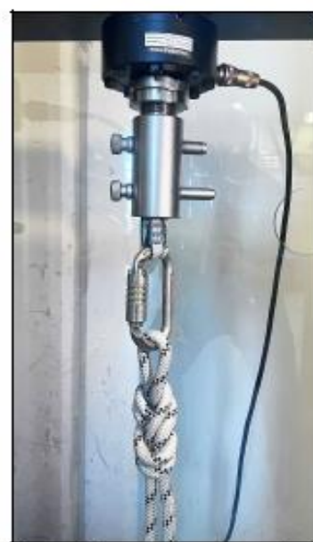
Figure 6. A typical setup for testing the tensile breaking strength of a knot, in this case a Figure Eight Loop. Photo credit: M. Goulet, courtesy Petzl® America.
