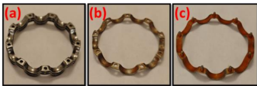
Figure 5. The cages of (a) healthy and (b, c) corroded specimens.
