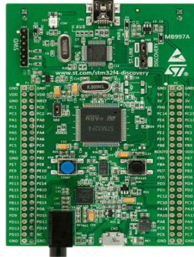
Figure 11. STM32F407 Discovery development board.
