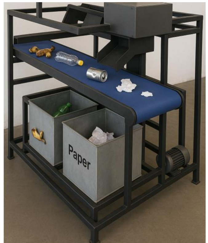
Figure 1: Assembled Low-Cost Automated Waste Sorting and Recycling System
