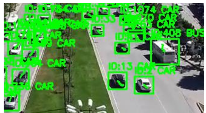
Fig. 14. Object Tracking with ByteTrack
