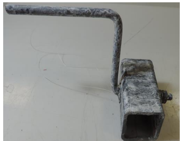
Figure 15. The appearance of the hook sets after the 96 th hour interim control
