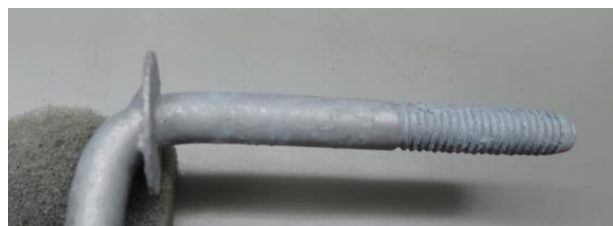
Figure 3. Appearance of unit-A before the salt spray test
