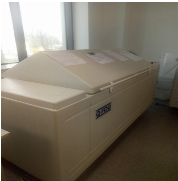
Figure 2. Salt spray test chamber
