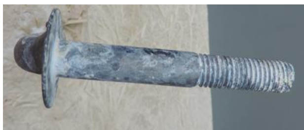
Figure 10. The appearance of unit-PD, after the 96 th hour
