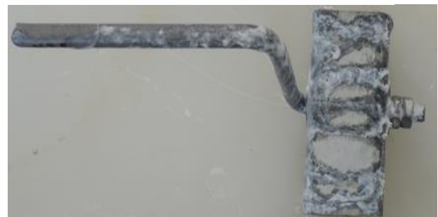
Figure 14. The appearance of the hook sets after the 72 nd hour interim control
