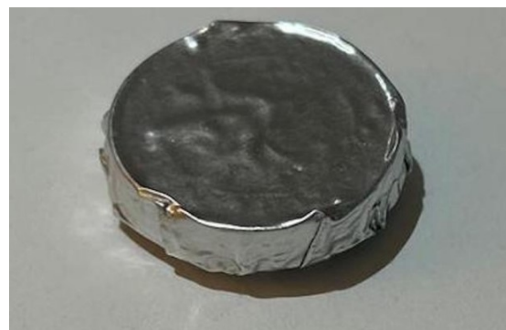
Figure 1: The metal cast model of 15 mm diameter and 6 mm height.
