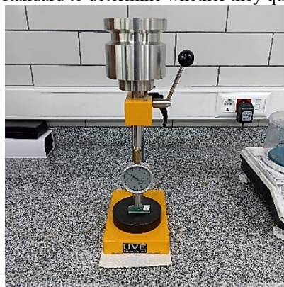
Figure 7. Shore D hardness tester (UVE Measurement Equipment) with Novotest durometer used for composite specimen hardness measurements.
