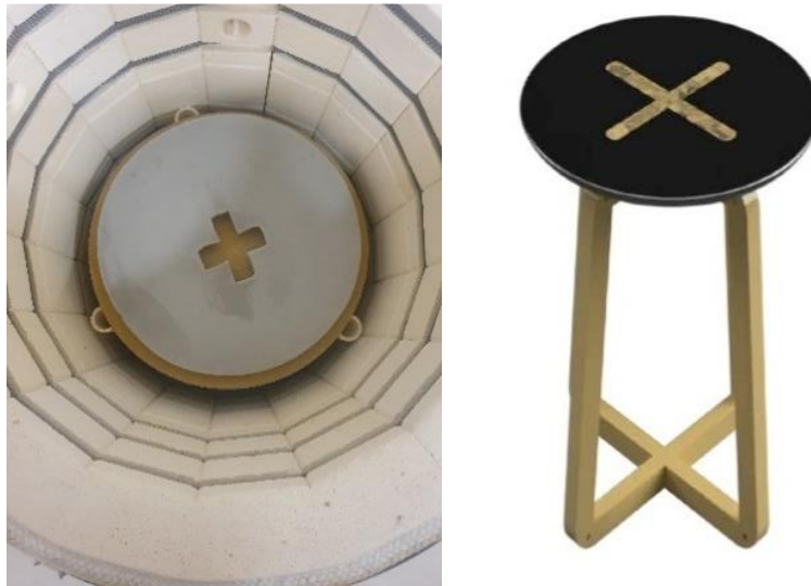
Figure 7. A student work before firing (on the left), which joins the top and the structure with a smaller central cross as it could cause breakage otherwise (on the right)
