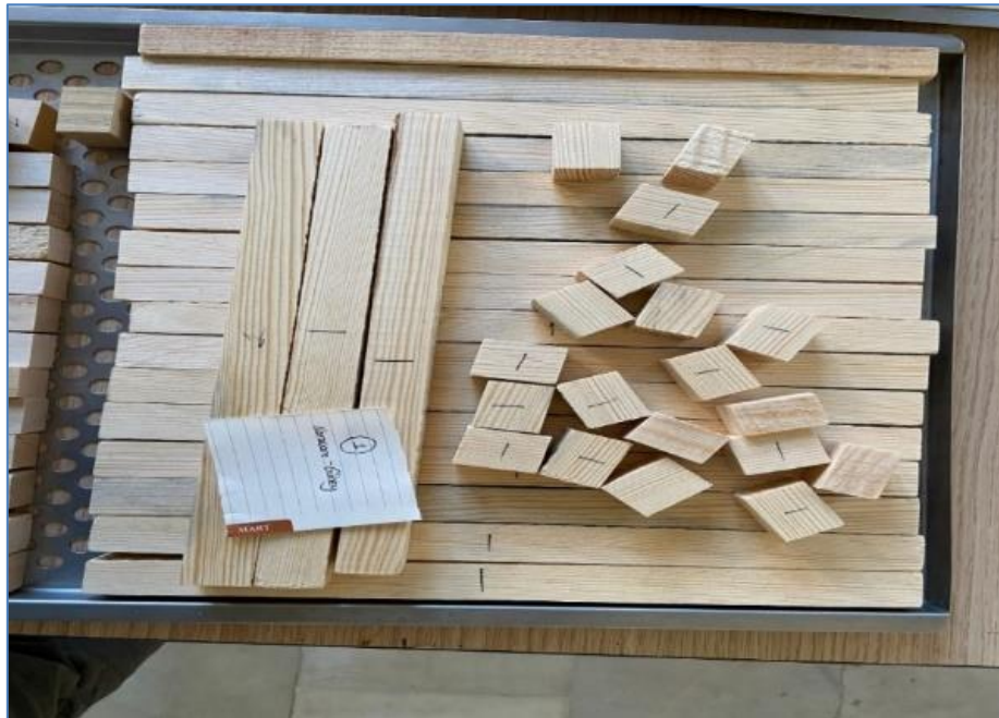
Figure 2. Density, bending strength, and compression strength test samples
