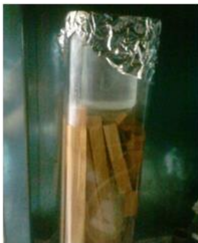
Figure 1. Beech wood samples impregnation into the acetic anhydride
