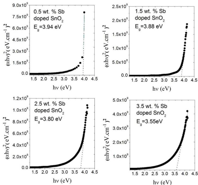
Figure 6.  $(\alpha hv)^2$ -versus  $h\nu$  spectra of Sb-incorporated  $\text{SnO}_2$  thin films.
