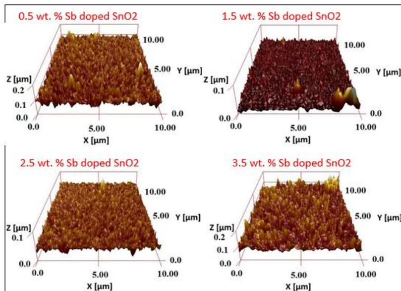
**Figure 4.** 3D AFM images of Sb-incorporated SnO<sub>2</sub> thin films.
