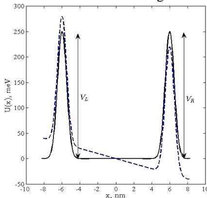
**Figure 1.** Potential profiles of Gaussian double barriers. The values of the parameters are given as  $V_L = V_R = 250$  meV,  $L_w = 6.0$  nm  $\sigma = 0.05$  nm. The solid line represents the potential profile of symmetrical GDB structure without electric field bias and dashed lines stand for case when the electric field ( $F = 50.0$  kV/cm) is applied.
