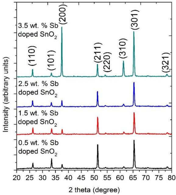
Figure 1. The XRD graphs of Sb incorporated SnO<sub>2</sub> thin films.
