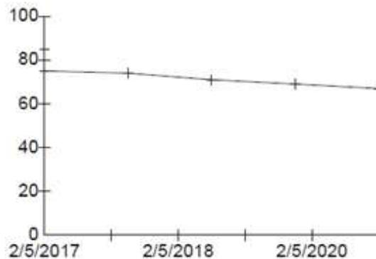
Graph 1. Section Condition Plot (Year vs. PCI).
