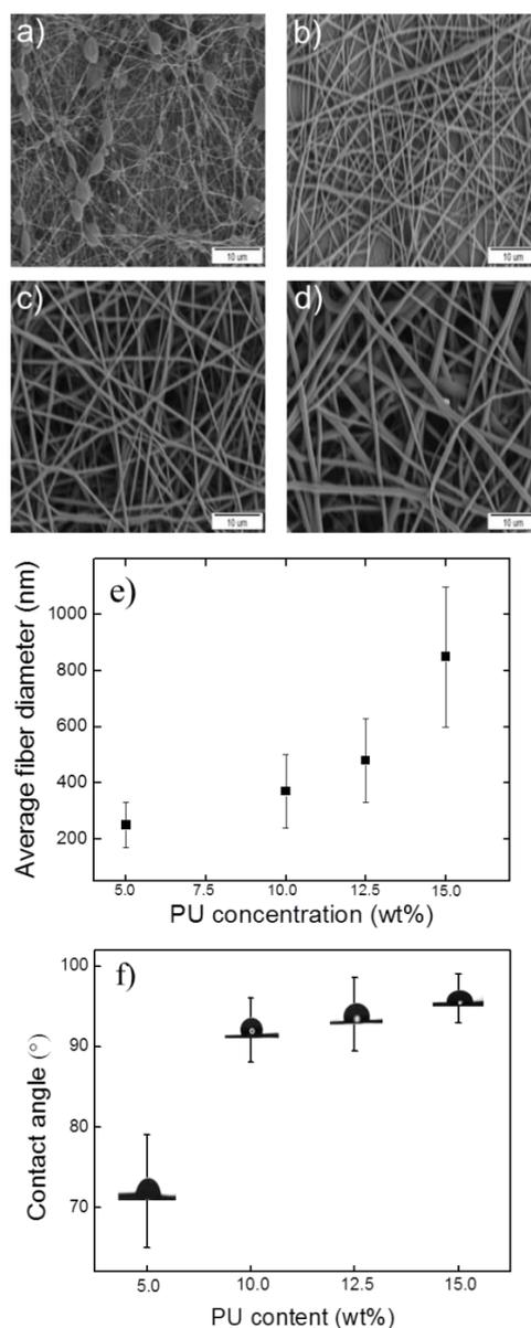
**Figure 1.** SEM micrographs of PU fibers obtained from electrospinning a) 5 wt% , b) 10 wt%, c) 12.5 wt%, and d) 15 wt% PU/DMF solutions. e) Average fiber diameter and f) contact angle of the fibers as functions of PU weight fraction. (Applied voltage: 12.5 kV, Flow rate: 1.00 mL/h, Distance: 17 cm).
