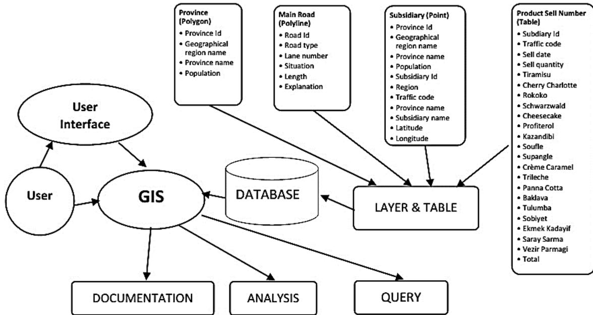
Figure 1. Schematic description of the created system.
