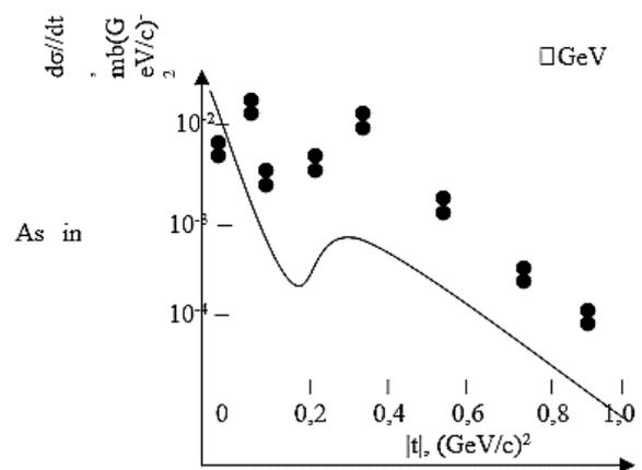
**Figure2.** Differential cross section for  $p^9\text{Be}$  scattering. The solid line corresponds to the cross-section calculated from equation (11), the points correspond to the experimental data from [12].
