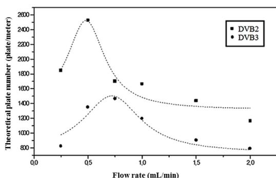
**Figure 5.** Variation of the theoretical plate number of the DVB2 and DVB3 columns with the flow rate (van Deemter diagram). Mobile phase: A: AcN / water. Analyte: Cytochrome C (0.25 mg / mL), Column dimensions: 100x4.6 mm ID., UV-VIS detector, 280 nm.
