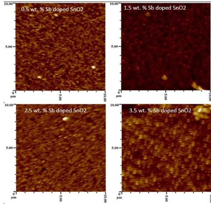
**Figure 3.** 2D AFM images of Sb-incorporated SnO<sub>2</sub> thin films.
