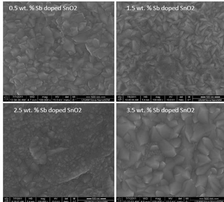
Figure 2. The SEM pictures of Sb-incorporated SnO<sub>2</sub> thin films.
