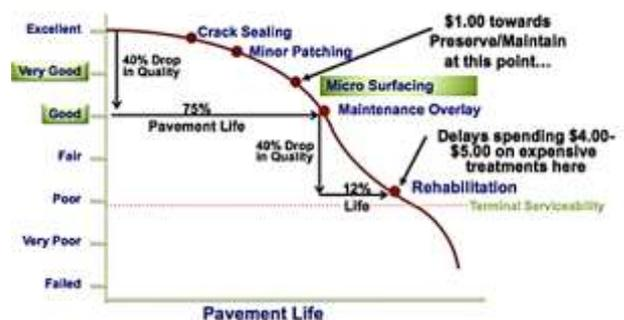
Figure 2. Pavement Condition Index (Cost Saving + Higher Service Level).
