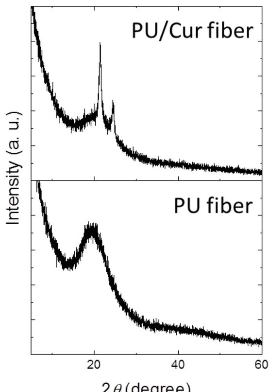
**Figure 3.** XRD patterns of of PU and PU/Cur fibers (PU content: 12.5 wt%, Cur content: 5 wt%, Applied voltage: 12.5 kV, Flow rate: 1.00 mL/h, Distance: 17 cm).
