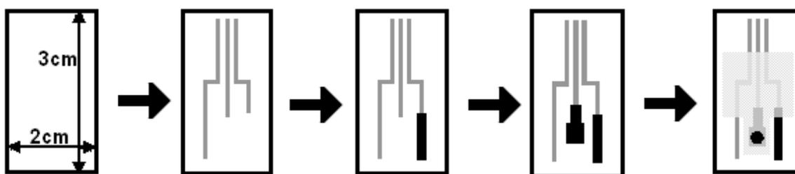
**Scheme 1.** 2 cm wide and 3 cm long electrode printing process contains printing of silver ink for pseudo-reference electrode and electrical contact layers (a), printing of counter(b) and working(c) electrodes by using carbon ink, and printing of insulating layer(d) by using the insulating ink respectively. Carbon ink of the working electrode contained 1%, 2% or 5% ratio of carbon nanotubes.
