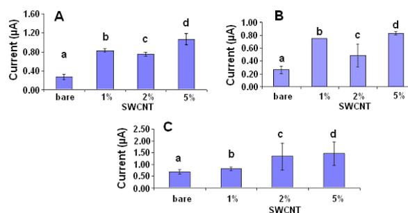
**Figure 1.** Graphs show the magnitude of guanine oxidation signals obtained from dsDNA immobilized surfaces (A) unpretreated CPE, (B) only 20s. ABS pretreated CPE (without potential application) (C) pretreated CPE applying at +1.7V potential during 20sec. and each column presents (a) bare electrode in the absence of carbon nanotube, (b) CNT-contained electrode in the presence of 1% SWCNTs, (c) 2% of SWCNTs and (d) 5% of SWCNTs modification onto CPEs.
