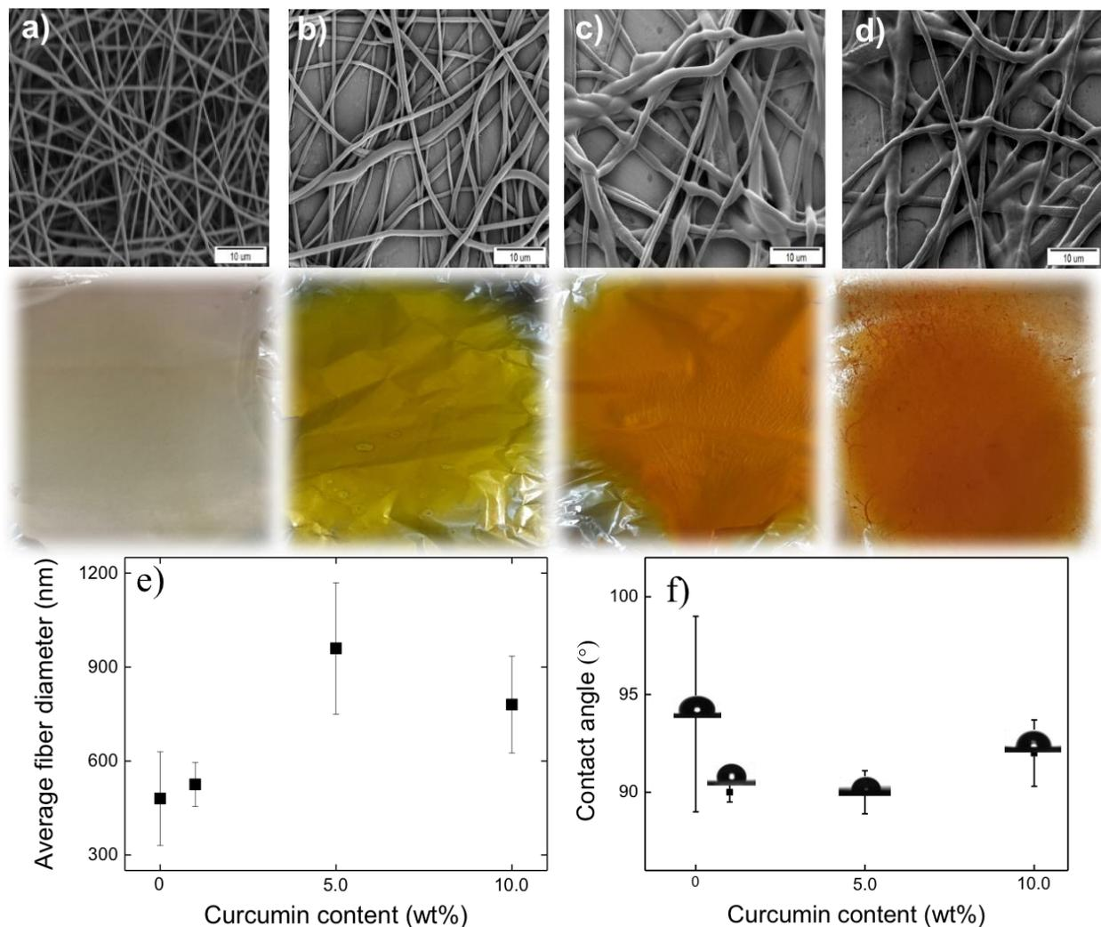
**Figure 2.** SEM micrographs and photographic images of the PU and PU/Cur fibers different curcumin concentrations a) 0 wt%, b) 1 wt%, c) 5 wt%, and d) 10 wt%. e) Average fiber diameter and f) contact angle of the fibers as functions of curcumin weight fraction. (Applied voltage: 12.5 kV, Flow rate: 1.00 mL/h, Distance: 17 cm, PU content in PU/Cur fibers: 12.5 wt%).
