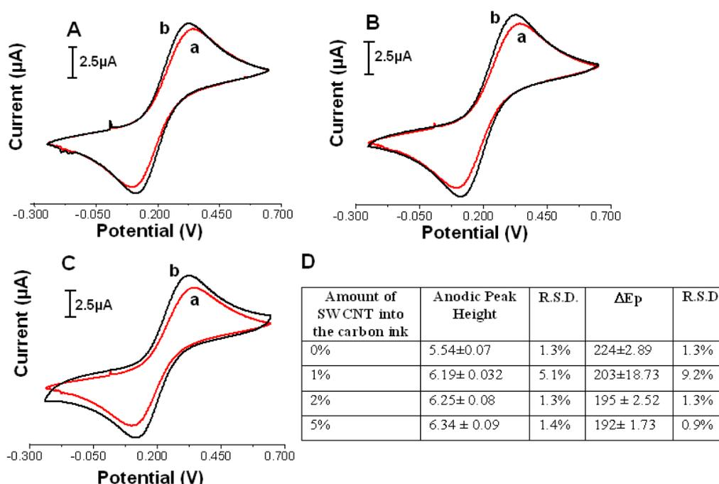
**Figure 2.** Cyclic voltammogram of 10 mM  $\text{K}_4[\text{Fe}(\text{CN})_6]/\text{K}_3[\text{Fe}(\text{CN})_6]$  (1 : 1) containing 1M KCl obtained from unpretreated bare (a) and SWCNTs-modified (b) SPE surfaces. The modification rates of SWCNTs in SPE are 1%(A), 2% (B) and 5%(C), respectively. The comparison of the electron transfer features of modified SPEs was also showed in the inset Table (D).
