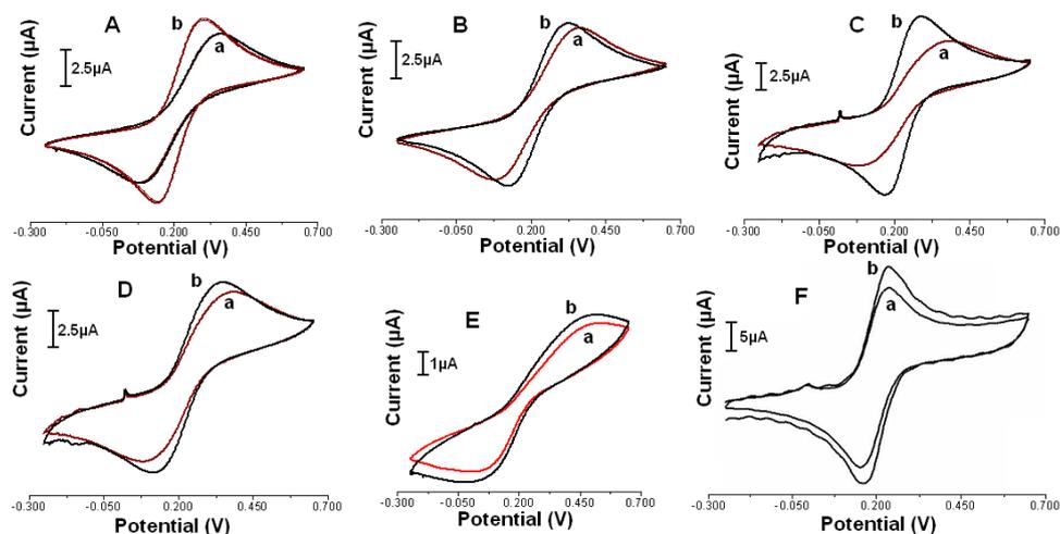
**Figure 5.** Voltammograms obtained from bare (a) and MWCNTs-contained (b) SPE surfaces with the solution of 10 mM  $K_4[Fe(CN)_6]/K_3[Fe(CN)_6]$  (1: 1) containing 1M KCl. The modifications of 2% ratio of bamboo(A,C, E and F) or hollow-structure(B and D) MWCNTs in SPE the surface of the SPEs were pretreated with  $H_2SO_4$  (A, B), acetone (C,D), Dimethylformamide(E) or NaOH (F). CV measurement parameters as similarly with the Figure 2.
