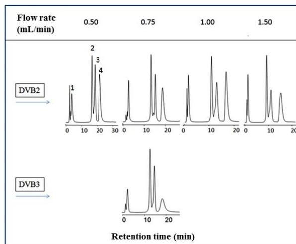
**Figure 4.** Sample chromatograms showing the effect of mobile phase flow rate on chromatographic separation of DVB2 and DVB3 columns in gradient conditions with RPC Flow rate (mL / min): 0.50, 0.75, 1.00, 1.50 Mobile phase: A: AcN + 5% water + 0.15% TFA B: Water + 0.15% TFA, Gradient conditions: 30% A to 60% B in 30 minutes in linear form. Column dimensions: 100x4.6 mm ID., UV-detector 280 nm. Peak order: (1) Ribonuclease A, (2) Cytochrome C, (3) Lysozyme, (4) BSA.
