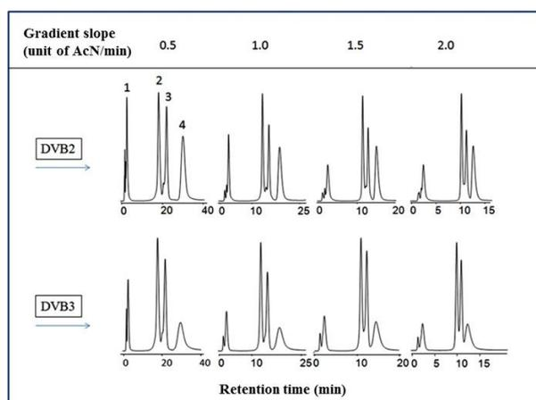
**Figure 3.** Sample chromatograms showing the effect of gradient slope on protein separation gradient conditions with RPC using DVB2 and DVB3 columns Flow rate (mL/min): 0.75 mL/min. Mobile phase A: AcN + 5% water + 0.15% TFA, Mobile phase B: Water + 0.15% TFA, Gradient conditions: 30% mobile phase A, 60% mobile phase B in linear form. Column dimensions: 100x4.6 mm ID., UV-detector 280 nm. Peak order: (1) Ribonuclease A, (2) Cytochrome C, (3) Lysozyme, (4) BSA.
