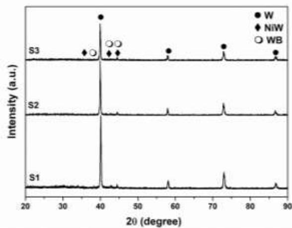
**Figure 3.** XRD patterns of the sintered samples.
