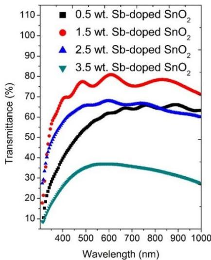
**Figure 5.** The optical transmittance spectra of Sb-incorporated SnO<sub>2</sub> thin films.
