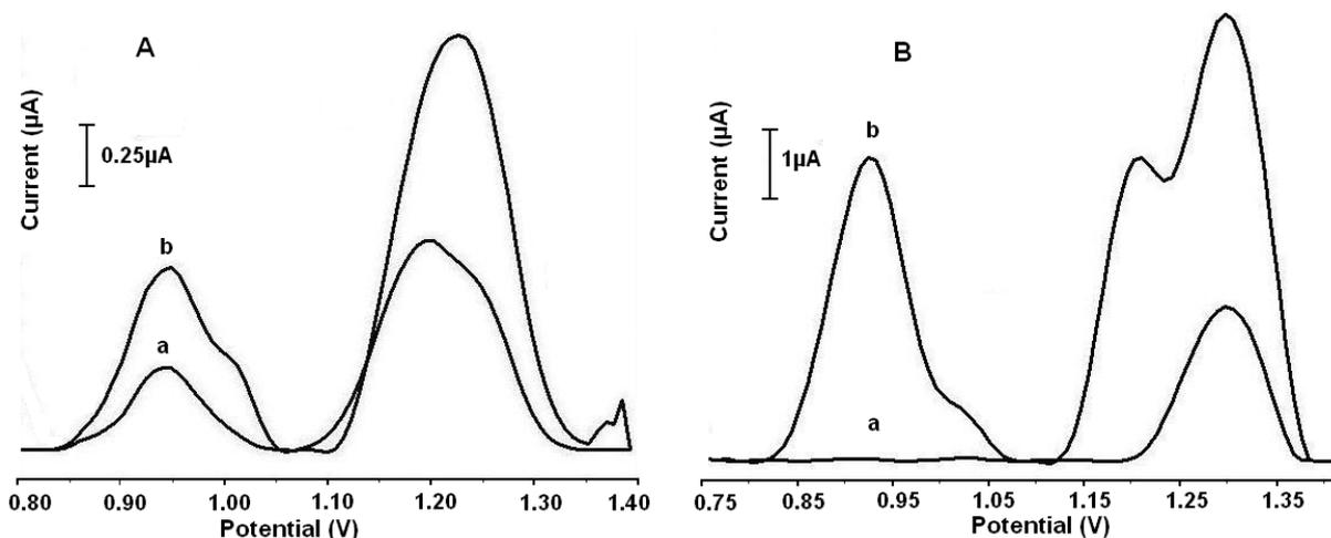
**Figure 6.** Influence of acetone (A) and NaOH(B)-based pretreatment process on the sensitivity of biosensor by using guanine-contained double stranded DNA. DPV of guanine oxidation signals obtained from DNA-modified bare (a) and bamboo-structured MWCNTs modified (b) electrodes.
