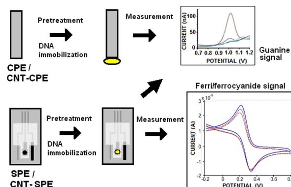
**Scheme 2.** Schematic diagrams illustrating the experimental steps of bare/CNTs-modified CPE and SPE electrodes and the detection of CNT-related signal enhancement based on guanine or ferri/ferrocyanide signals.
